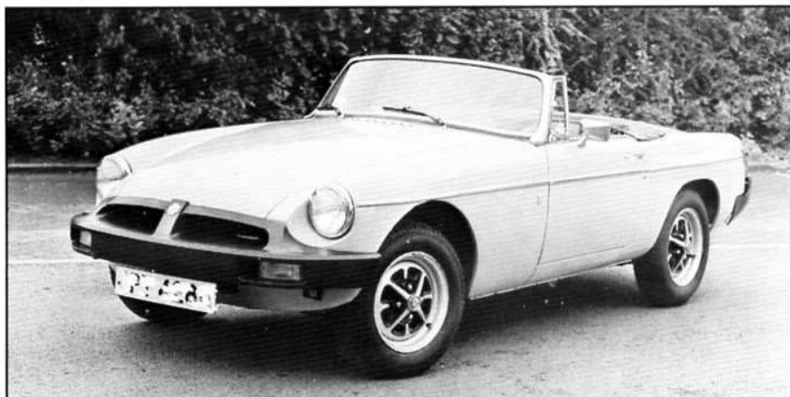
MGB Roadster in 1974 with rubber bumpers and increased ride height, changes that no-one at Abingdon wanted but which were forced upon MG by external influences
