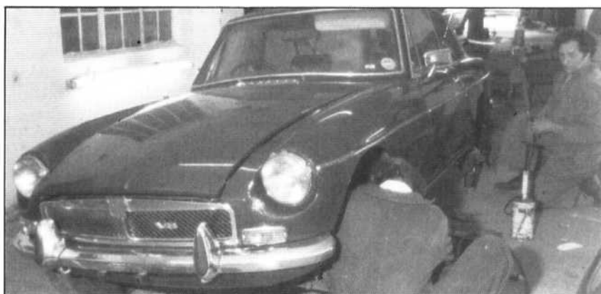
Below, applying the finishing touches to the car at the workshops of R H Smart in Swavesey, where it received a complete and thorough body refurbishment including a windows-out respray and the replacement of several body panels
