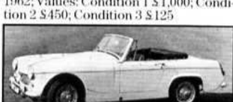
Model Midget MkII 1964-1966 Number prod 26,601; Capacity 1098cc; Power 59bhp; Top Speed 91.8mph; 0-60mph 14.9sec; Av fuel con 29.2mpg; Tested 1964; Values: Condition 1 $1,925; Condition 2 $875; Condition 3 $425
