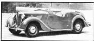
Model Y-Type or 1/4-litre 1947-1953 Number prod 8336; Capacity 1250cc; Power 46bhp; Top Speed 70mph; 0-60mph 29.3sec; Av fuel con 30mpg; Tested 1951; Values: Condition 1 $2,675; Condition 2 $1,725; Condition 3 $650
