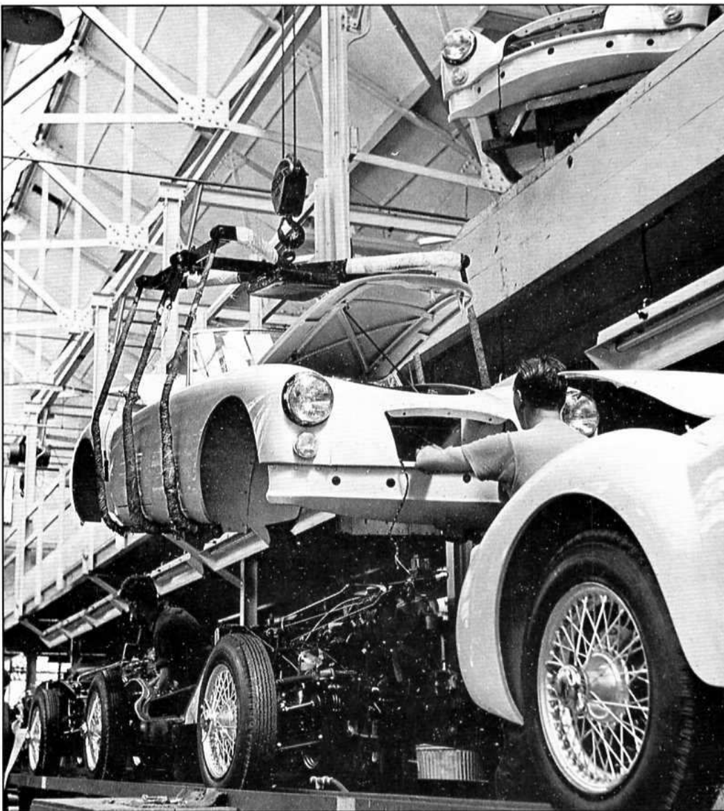
A shot taken in 1960 but looking more recent, showing MGAs having their bodies fitted on the production line at Abingdon
