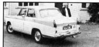
Model Magnette MkIV 1961-1968 Number prod 13,738; Capacity 1622cc; Power 68bhp; Top Speed 87.5mph; 0-60mph 17.3sec; Av fuel con 25.2mpg; Tested 1962; Values: Condition 1 $1,350; Condition 2 $745; Condition 3 $200
