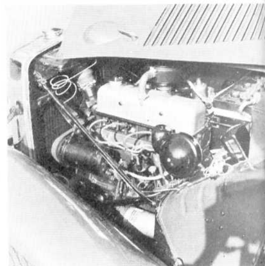
Above, the XPAG 1250cc engine of the TD, the basic unit that also powered the TC and TF.
