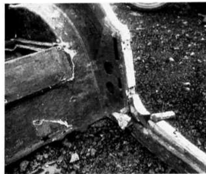
Top, clockwise, replica parts, the front suspension link of the TD/F; the state that the wooden frame can get in; they really can deteriorate in this way; a replica body by Naylor Brothers; close up of rot point, note glass fibre disguise of rear bulkhead corrosion.
