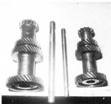
What a contrast, TC layshaft (left) and weaker TD/F shaft (right). Not surprisingly the latter gives trouble.
