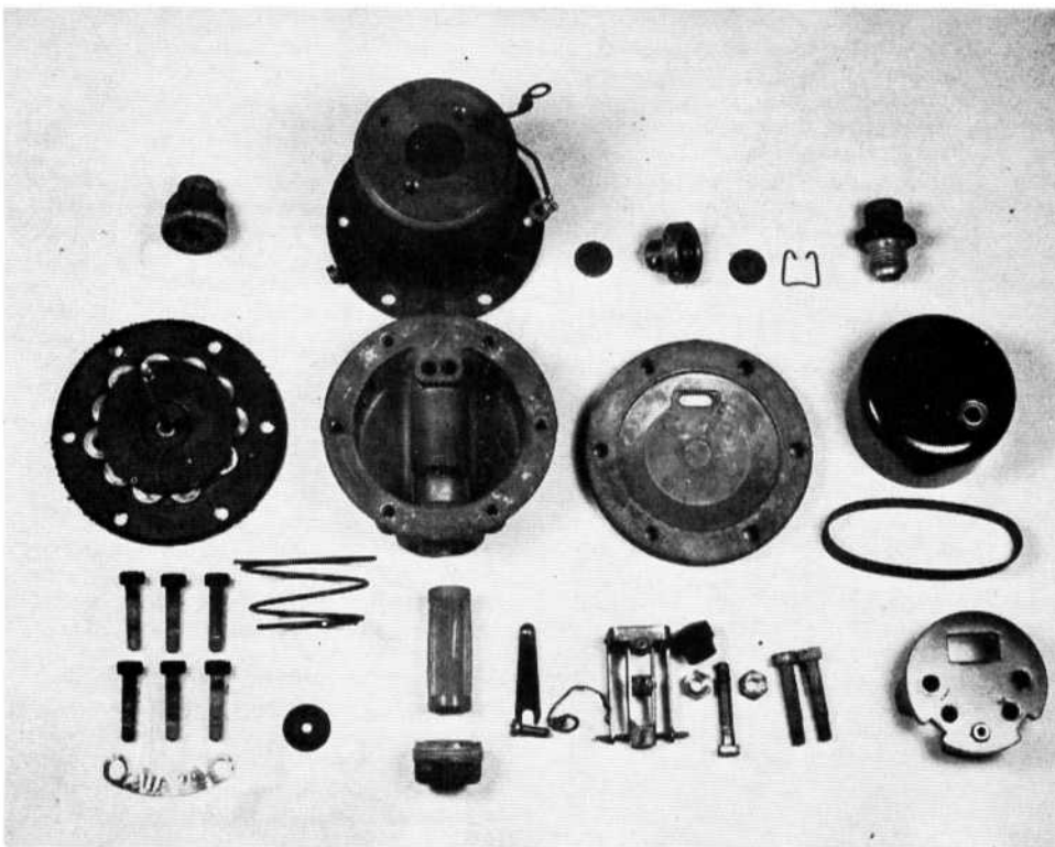
An older L type pump stripped down. From left to right, the top row is: inlet union, solenoid body, inlet valve, outlet valve cage, outlet valve, spring clip, outlet union. Middle row: diaphragm with rollers, pump body, sandwich plate, end cap and rubber dust ring.
