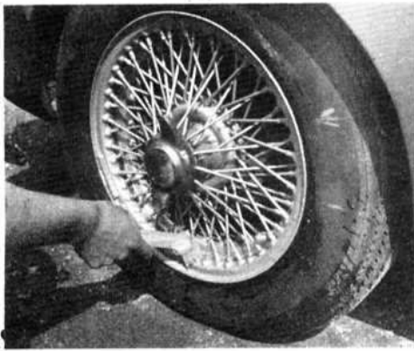
Far left, wheel rebuilt by Motor Wheel Services. Above left, weekly care – clean with small stiff brush. Above centre, check spokes with wheels off the ground for tightness. Above right, with tyre off, check rim and spoke ends.
