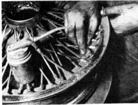
Above left, clean spoke and adjusters with wire wool and oil. Above centre, fit new rim tape. Above right, adjustment by experts (Motor Wheel Services). Right, properly maintained the wire wheel looks good, is reliable and safe.
