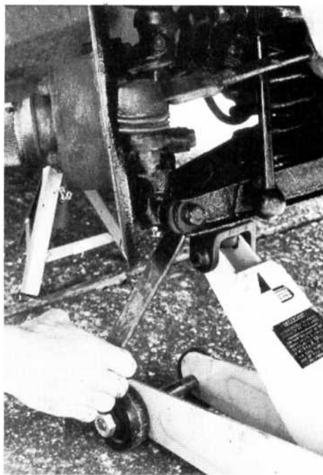
The trunnion bolt had been turning in the ends of the wishbone arms and worn the holes oval. New arms were not quickly available, so the holes were welded up and redrilled.
