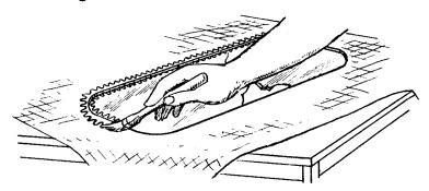
2) Cut patch of hood material to overlap damaged backlight by 1" (25.4 mm.) all round and, with hood flat, stitch patch to inside of hood, the stitch-line being  $\frac{7}{3}$ " (.875" or 22.22 mm.) from the light opening:
