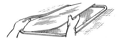
5) Stitch through centre of remaining portion of damaged backlight, hood-cover, new backlight and patch, then cut patch level with light opening:
