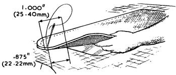
3) Cut damaged backlight flush with light opening, leaving portion welded to hood intact:
