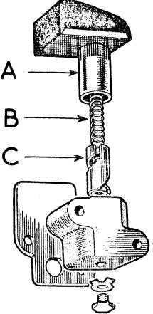
The slipper head assembly of the timing chain tensioner fitted to the above is now offered as a service part under Part No. 17H31.
