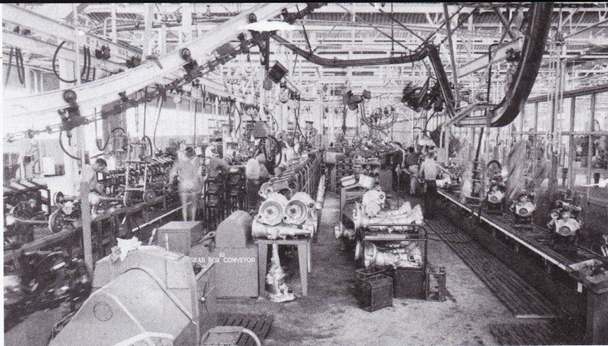
ABOVE: The final assembly of major mechanical components took place at Zetland, and here we can see (from left to right) rear axles, gearboxes and engines.
