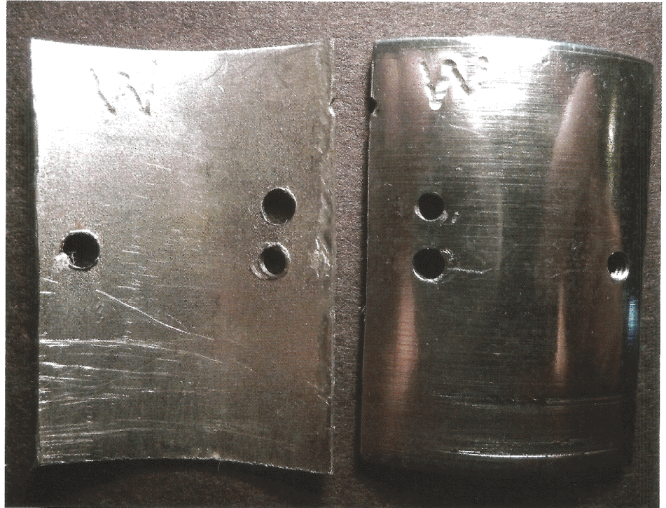
The mild steel and section of float chamber before entering the container
