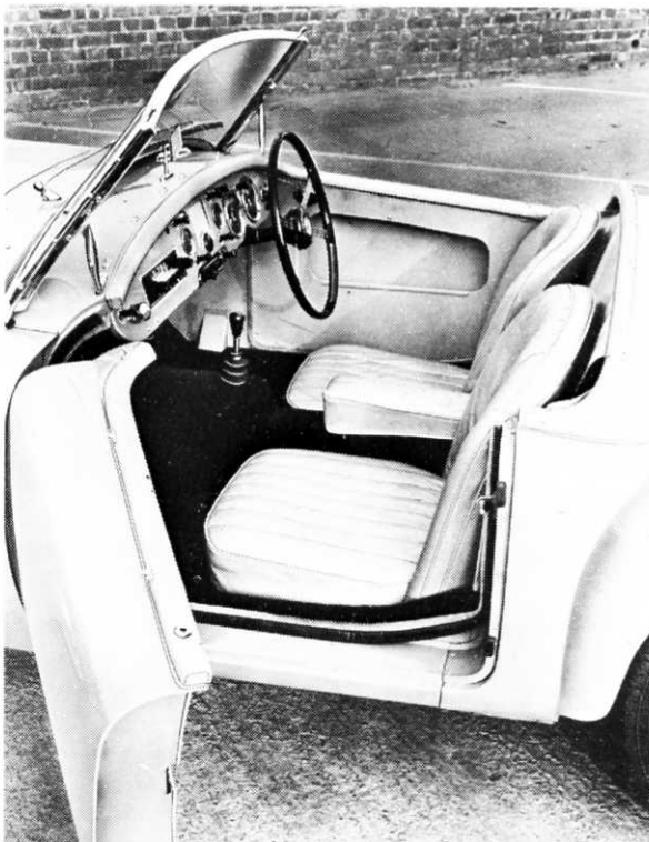
Seats tip forward if required. Instruments confront the driver but the horn is in the centre of the fascia
