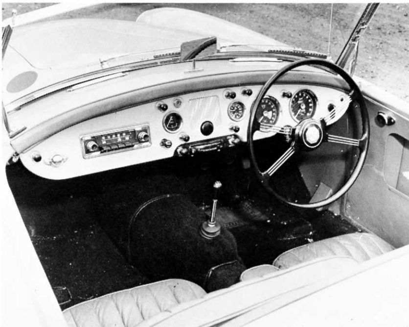
Instruments on the fascia include speedometer, rev counter, water thermometer, oil pressure gauge and fuel gauge. On the extreme left there is a map-reading light
