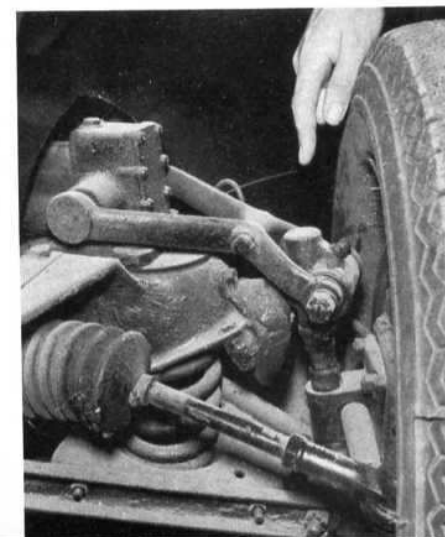
Below, check for suspension wear by wobbling jacked-up wheel.
