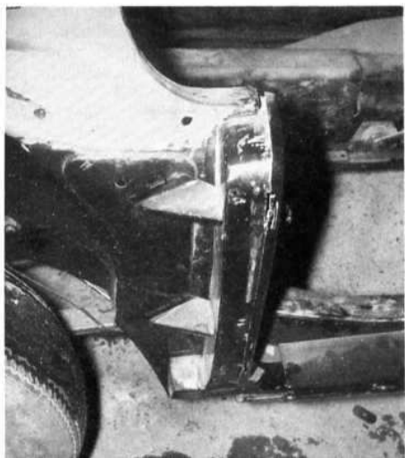
Above, rot in chassis side member; below, door shut face showing rust traps.
