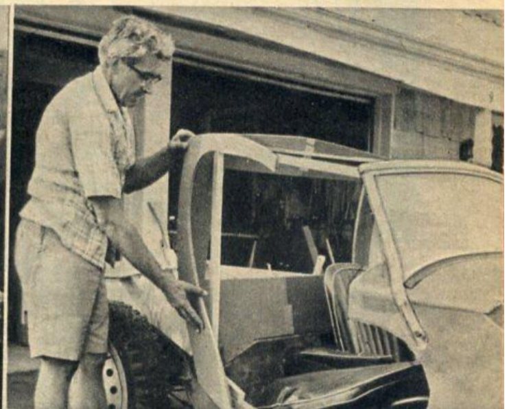
PLYFOAM body section is attached temporarily to wooden frame before glassing.
