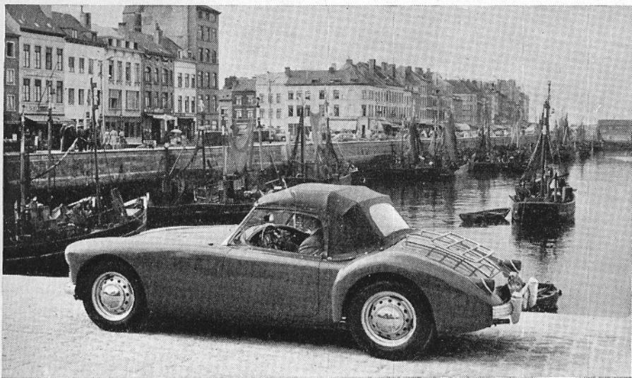
Less noise but still quite good weather protection is obtained with hood up and side-screens stowed away. Visibility to the rear is reasonable through a wide plastics window.
