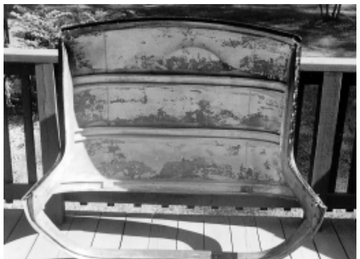
Stripped hardtop with some glue still to be removed
