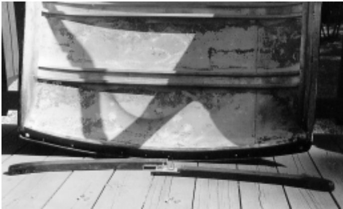
The method of splitting and rejoining the front bow.
