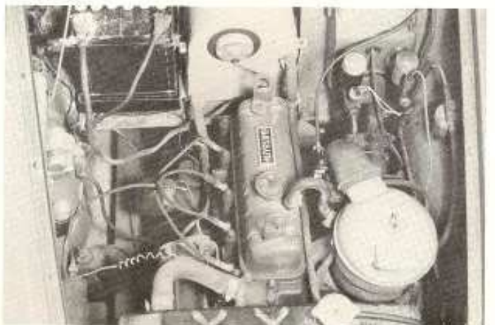
The engine was manufactured under license from Austin, and should be familiar to any BMC fans. The carbon pile voltage regulator is located next to the ever-present "Under Hood Light".
